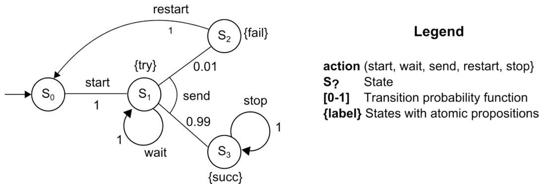
Figure 8: Markov decision process model of a simple communication protocol (Parker, 2011)
