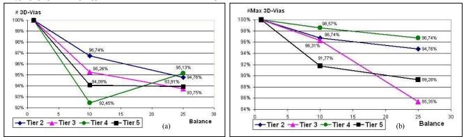
Figure 3. Evolution of the number of 3D-Vias obtained with the unbalance of the I/O paritioning process.
