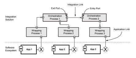
Figure 1. A typical EAI solution.
