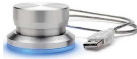
Fig. 2: USB controller (PowerMate, Griffin Technology) used to rate the level of fun.
